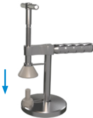
Fig. 49 Mount the Prosthesis Head Adapter Support onto the Press (Fig. 49).
